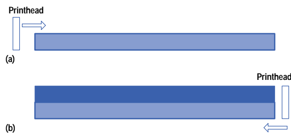
Fig. 6. (a) In making the transition from Blank Skipping to Black Text Printing , the printer prints the first pass of the black text region with the bottom half of the printhead, advances the paper half a printhead height, and then enters the Black Text Printing state. (b) During the next sweep generated, the Black Text Printing state finishes the lines that were printed during the transition and continues printing the black text region.
